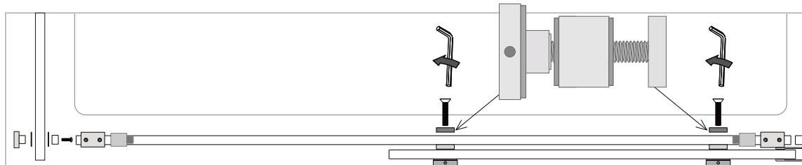
Install the anti-collision block onto the guide rail first,
