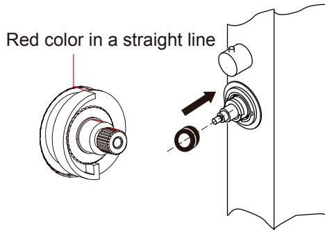
④ Press the button on the head and put on the head as below ensuring the screw hole pointing to the front
