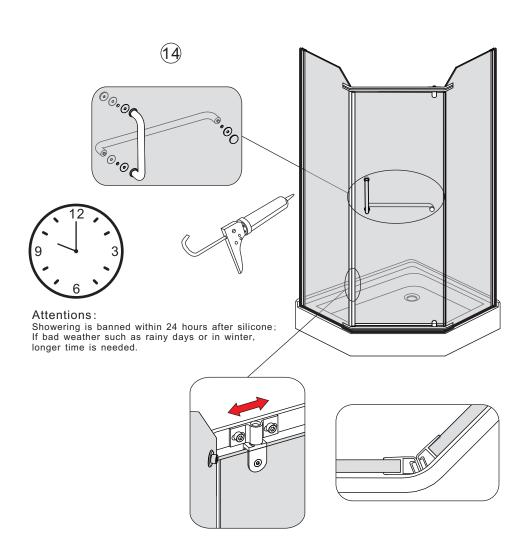
When magnet strips on the door are not aligned, please adjust the pivot, make sure that magnet strips attract each other well.
