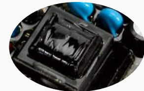
Gluing treatment, waterproof upgrade
